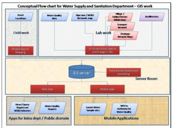
The highlight of the effort was the method of mapping the WSS schemes using traverse method of GPS with the air valve as reference. Mapping of pipelines is very difficult and tedious job as pipeline survey is to be carried out by traversing on the pipeline.
